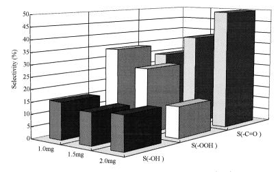
Fig. 5. Effect of the catalyst amount on oxidation of cyclohexene (1 ml) at 343 K.
