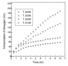
Fig. 2. Relationship between consumption of  $O_2$  with reaction time catalyzed by Sal–Phe–Mn in different temperature (Cat: 2 mg; Sub: cyclohexene (2 ml)).
