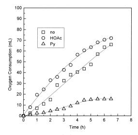
Fig. 3. Effect of the additive (5%) in the oxidation of cyclohexene (1 ml) in the presence of Sal-Phe-Mn (1 mg) at 343 K.
