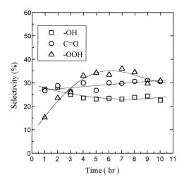
Fig. 1. Relationship between the selectivity of the major products and reaction time (Cat: 2 mg; cyclohexene: 3 ml; 343 K).
