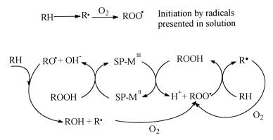
Fig. 4. The allylic peroxide decomposition mechanism for dioxygen reactions with metal complex (SP-M = Sal–Phe–Mn). Initiated by radicals in solution, the peroxides thereby generated are catalytically decomposed by the manganese complex. These radicals can then propagate the reaction further.
